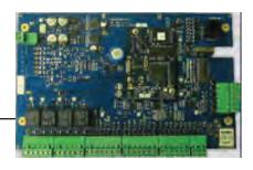
The PRO3000 combines intelligent controller and reader interface into one complete unit. It connects for two readers via Wiegand controlling two doors. The controller can support up to 62 doors via RS485 multi-drop communication where 30 downstream controllers are connected to the gateway controller. This architecture can reduce the usage on LANs by using only one TCP/IP address to 62 doors.
